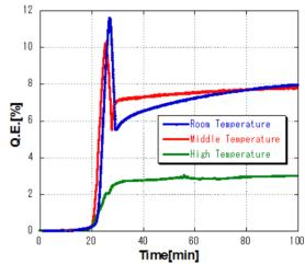
Figure 4: Q.E. measurement during Cs deposition.
