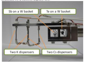
Figure 2: New-designed evaporation source holder.
