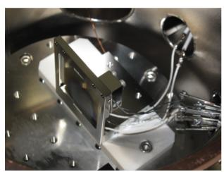
Figure 3: A substrate heating system.
