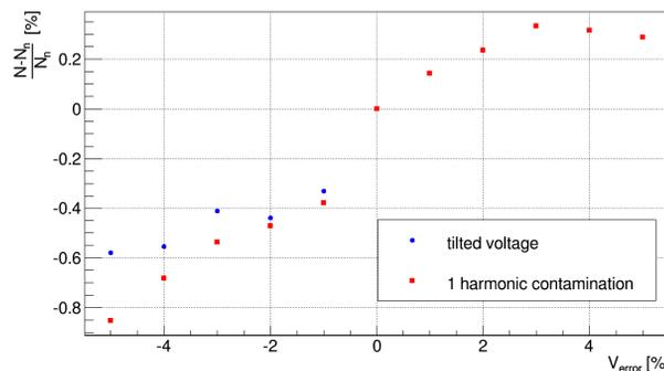
Figure 4: relative transmission vs voltage error. Tilt and one harmonic contamination are shown.
