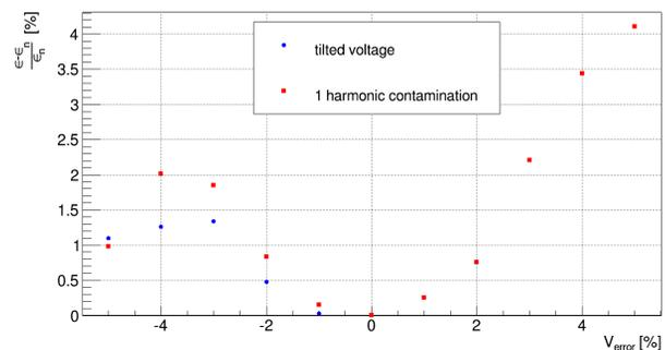
Figure 5: relative longitudinal rms emittance growth vs voltage error. Tilt and one harmonic contamination is shown.
