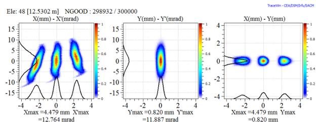
Figure 3: Phase space at the HRMS image point. The three beams are separated of 1/20000 with  $\pm 1$ eV energy spread.
