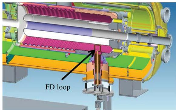
Figure 3: Cross section view of the 56 MHz cavity cryomodule with the FMD fully inserted.
