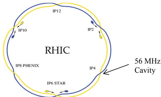
Figure 1: Location of the 56 MHz cavity in RHIC.
