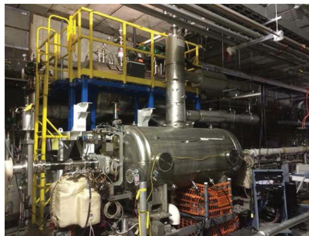
Figure 5: The 56 MHz cryomodule in RHIC tunnel.
