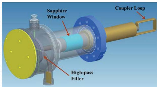
Figure 4: The HOM coupler with high pass filter for 56 MHz cavity.
