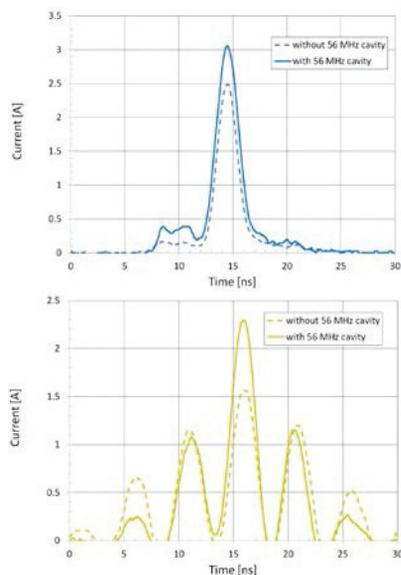
Figure 7: Beam profile comparison for 56 MHz cavity turned on and off. Top: Blue ring with He<sub>3</sub> particles. Bottom: Yellow ring with Au particles.
