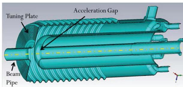
Figure 2: Cross-section view of the 56 MHz SRF cavity.
