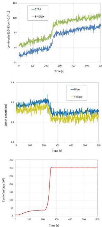
Figure 6: Luminosity increase and bunch length decrease due to the 56 MHz cavity turned on.
