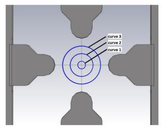
Figure 5: Radial position of the curves for multipole components analyses.
