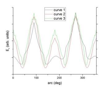
Figure 6: The radial E-field along the curves at the stem for the x-electrodes (position a).
