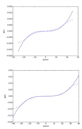
Figure 2: The magnetic field profiles with the minimum (top) and maximum (bottom) distance (dash line) between the two C-type dipoles compared with octupole (solid line).
