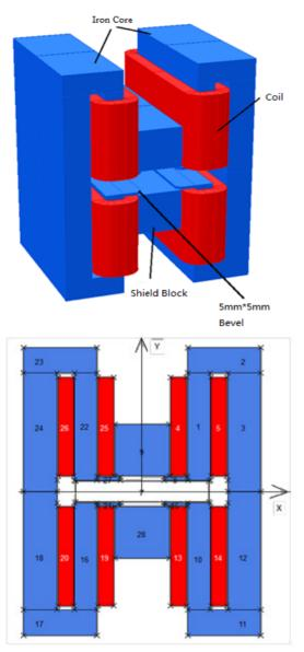
Figure 1: The 3D model of the new type of magnet (top) and the central plane of the magnet (bottom).
