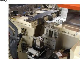
Figure 8: The reference laser is set on pedestal for recalibration.
