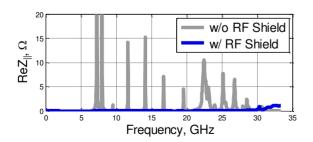
Figure 6: Real Part of the Longitudinal Impedance.
