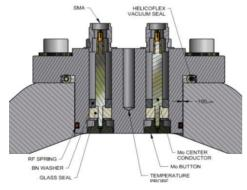
Figure 1: BPM Flange fixed to vacuum vessel. The clearance of the BPM Flange ~100µm from the contact vacuum chamber surface.
