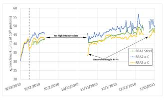
Figure 6: The daily fit of the  $x_0$  benchmark is shown over time for RFA1 (steel), RFA2 (a-C near steel), and RFA3 (a-C). After a vacuum leak occurs (dashed line) near to RFA3, the  $x_0$  benchmark for RFA3 decreases dramatically and lags behind RFA2.
