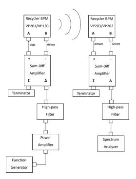
Figure 1: Flow-chart schematic of the microwave electron cloud measurement. The signal generator creates a signal at a single carrier frequency, next this signal propagates through the electron cloud, and lastly this signal is examined for phase modulation in the signal analyzer.
