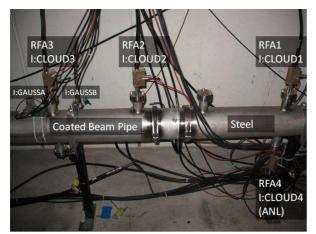
Figure 5: The electron cloud measurement setup in the Main Injector at MI-52. The setup primarily consists of four RFAs and two beampipe sections. The beampipe is 6" in diameter and the coated and uncoated sections are each  $\sim 1$  meter long. The setup is located in a straight section to avoid electron confinement from magnets.
