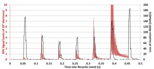
Figure 4: Signals from an RFA (red) measured in volts and a typical loss monitor (black) over the Recycler cycle.
