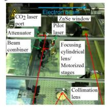
Figure 4: Laser and optical system of the CBS setup.
