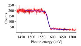
Figure 8: Zoom into Compton edge of Fig. 6 (b) and curve fitting at 1.3 GeV,  $\chi^2/\text{ndf} = 524/555$ .
