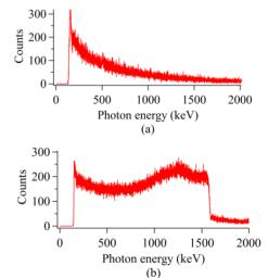
Figure 6: Spectrum at 1.3 GeV for over 120 seconds: (a) radiation background (laser off, e beam ~10.7 mA); (b) CBS signal + background (laser on, e beam ~9.3 mA).
