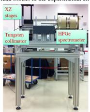
Figure 3: Gamma ray detection system.
