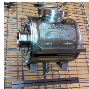
Solenoid installed in He vessel
