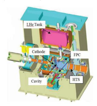
Figure 1: ERL SRF gun cryomodule.
