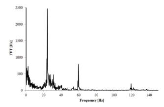
Figure 4: FFT microphonics spectrum.
