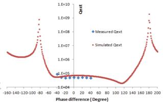
Figure 7: Comparison of measured external *Q* factor and simulation results.
