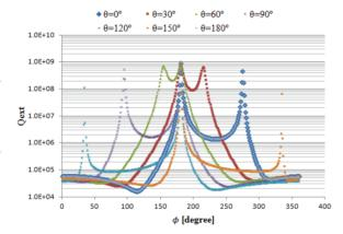
Figure 6: The external *Q* factor change with one phase shifter at different initial states.
