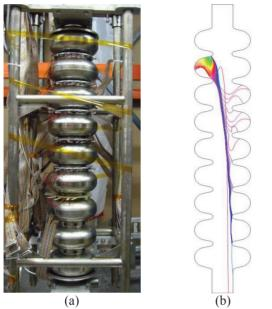
Figure 1: (a) A nine cell ILC cavity equipped with cryogenic radiation detection diodes for field emitter localization; (b) Trajectories of electrons emitted from the location as determined by the JLab procedure.
