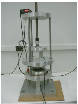
Figure 1: Dumbbell measuring fixture with a dumbbell under test, the applied force is 295 pounds.
