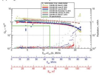
Figure 3: SSR1 bare cavity test performance.
