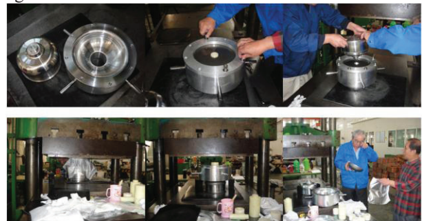
Figure 4: Deep drawing of the half-cell.
