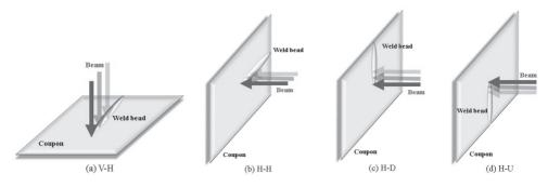
Figure 1: Schematic layouts of combinations of a generator position and a welding direction. (a) V-H: the vertical generator position and the horizontal welding direction, (b) H-H: the horizontal generator position and the horizontal welding direction. (c) H-D: the horizontal generator position and the downward welding direction, and (d) H-U: the horizontal generator position and the upward welding direction.
