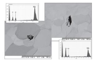
Figure 4: Examples of contaminants found after the BCP [3]. The contaminants include carbon and oxygen, or carbon, nitrogen and oxygen.
