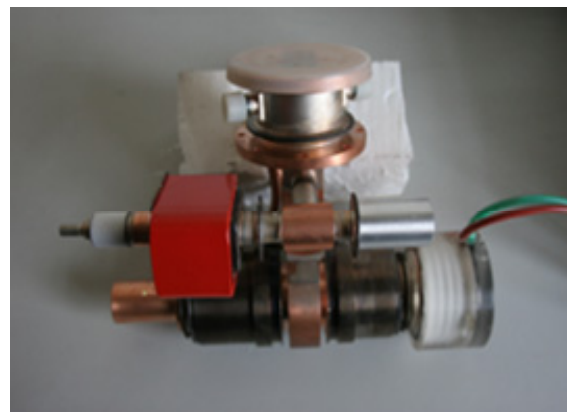
Figure 2: Photo of the fully sealed accelerating tube after Welding.
