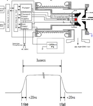
Figure 1: The gun structure (top) and the gun beam pulse form (bottom).
