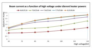
Figure 7: Beam current vs. high voltage.
