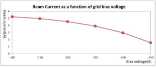
Figure 8: Beam current vs. grid bias voltage.
