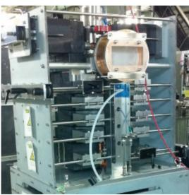
Figure 3: The magnets have larger aperture than the klystron body before the klystron installation (top). After the klystron installation, the magnets are brought close to the klystron (bottom)
