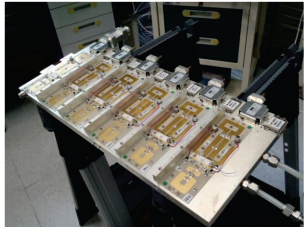
Figure 5: One of three wings supporting 6 innovative, fully planar RF modules developed at the ESRF.
