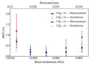
Figure 5: RDT vs. beam momentum offset for sextupolar and octupolar resonances for the standard PS configuration at 14 GeV/c. Both measurements and simulations results are shown for the sake of comparison. The measured tune is reported in the second horizontal scale.
