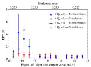
Figure 4: RDT vs. figure-of-eight loop current variation for sextupolar and octupolar resonances for the standard PS configuration at 14 GeV/c. Both measurements and simulations results are shown for the sake of comparison. The measured tune is reported in the second horizontal scale.
