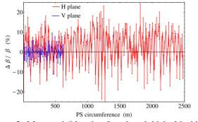
Figure 2: Measured  $\beta$ -beating for a bunch kicked inside a stable island generated at 14 GeV/*c* (The PS circumference is  $2 \pi 100$  m long).
