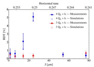
Figure 3: RDT vs. J for sextupolar and octupolar resonances for the standard PS configuration at 14 GeV/c. Both measurements and simulations results are shown for the sake of comparison. The measured tune is reported in the second horizontal scale.
