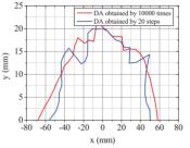
Figure 6: DAs obtained by the step-by-step chromaticity compensation method (blue line) and Method 1 (red line).
