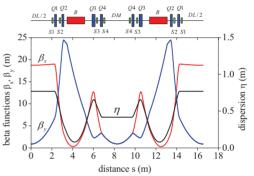
Figure 2: The magnet layout and linear optics functions of one period of the studied lattice.
