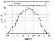
Figure 8: DAs obtained by Method 3 (black line) and optimizing sextupole strengths using PSO (red line).
