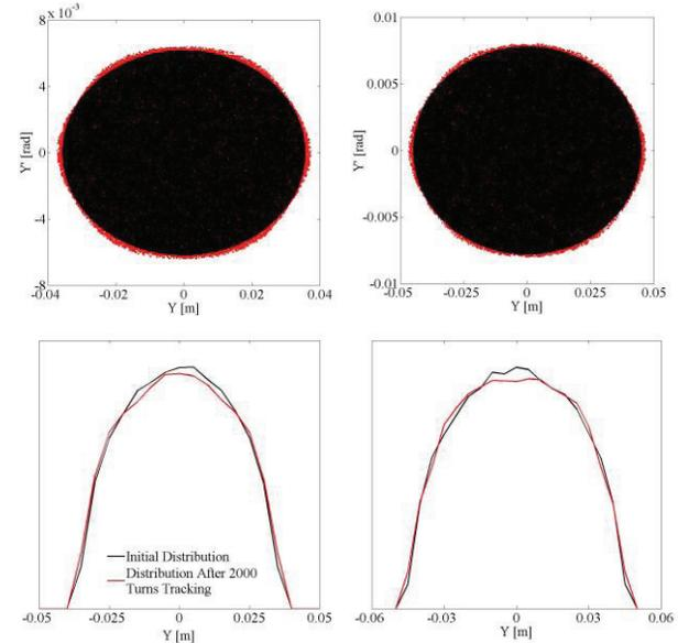
Figure 4: The effects of the chromaticity sextupoles on the beam distribution; the left figures are the simulation results for the case of with the initial emittance of  $220\pi$ -mm-mrad, and the left figures are the simulation results for the case of with the initial emittance of  $350\pi$ -mm-mrad; the black dots indicate the initial distribution, and the red dots indicate the distribution after 2000 turns tracking.
