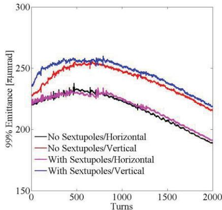
Figure 5: The 99% emittance evolutions during acceleration with and without chromaticity sextupoles.
