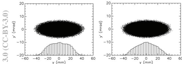
Figure 6: The painted distributions in vertical direction with (right) and without (left) chromaticity sextupoles.
