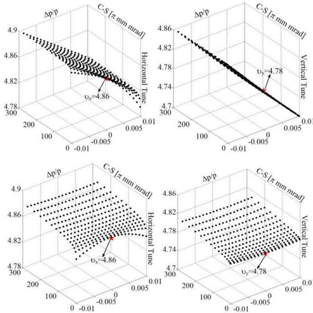
Figure3: Betatron tunes for particles with different momentum spreads and Courant-Snyder (C-S) invariants with (bottom) and without (top) chromaticity sextupoles.
