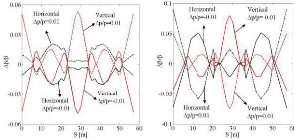
Figure 2: The dependence of the Beta functions on the momentum spread along a super-period with (right) and without (left) chromatic correction ( $\Delta\beta = \beta_{\Delta p \neq 0} - \beta_{\Delta p = 0}$ ).
