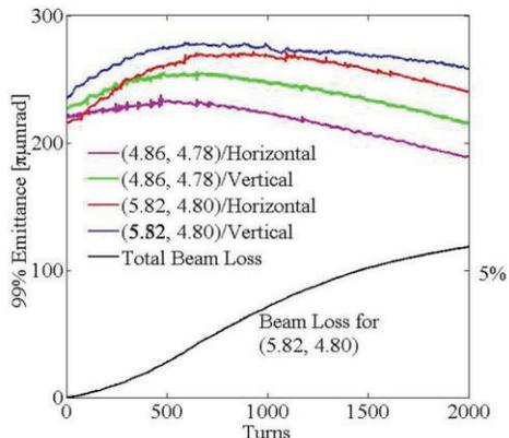
Figure 5: The 99% emittance evolution and beam loss during acceleration.
