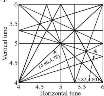
Figure 1: Working points of (4.86, 4.78), (5.82, 4.80) in tune space; up to fourth order structure resonances are shown.
