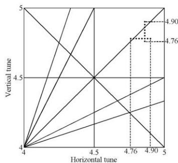
Figure 3: Investigated working points near the tune (4.86, 4.78) in tune space; up to fourth order structure resonances and half integer resonances are shown.
