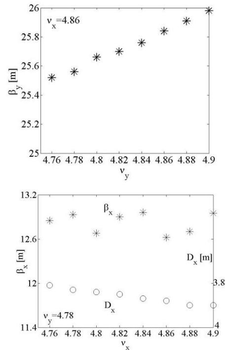
Figure 4: The comparison of the maxima of beta functions and dispersion functions for different working points near the tune (4.86, 4.78).
