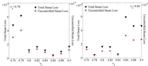
Figure 6: The beam loss during the 2000 turns tracking for working points near (4.86, 4.78).
