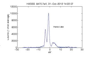
©Figure 6: An iSASE FEL spectrum with undulator in Fig. 5.
