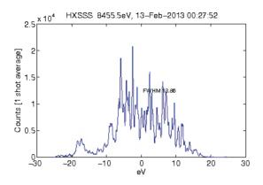
Figure 4: A SASE FEL spectrum with undulator in Fig. 3.
