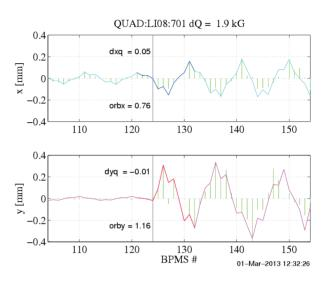
Figure 1: Quad shunt technique. A quadrupole at the location of the vertical line is changed and the resulting orbit change is fitted with a kick (blue and red), the cyan and magenta parts are extrapolations.
