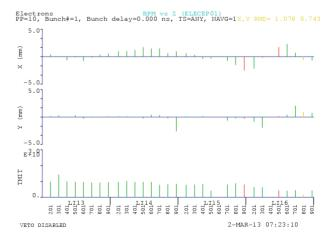
Figure 7: Ballistic orbit (all off) in Li14 to Li16.
