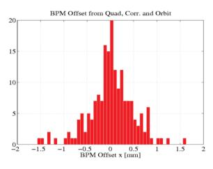
Figure 3: Distribution of the BPM offsets in x calculated from the strengths of quads, correctors and the orbit.
