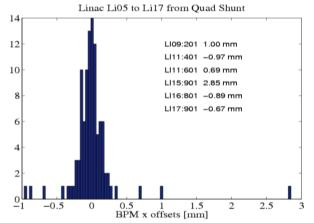
Figure 2: Distribution of the horizontal BPM to quadrupole offsets from quad-shunting.
