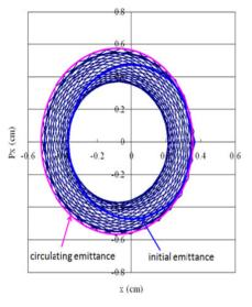
Figure 1: At 1MeV, the circulating emittance produced by phase space filling up due to the first harmonic field error simulated by CYCLONE.
