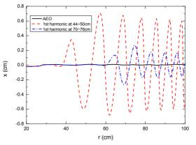
Figure 2: The radial coherent oscillations due to the first harmonic field error at different radius range.
