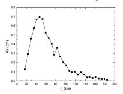
Figure 3: The coherent oscillation amplitudes excited by a the first harmonic field bumps, which are Gaussian shaped, at different radius ranges.
