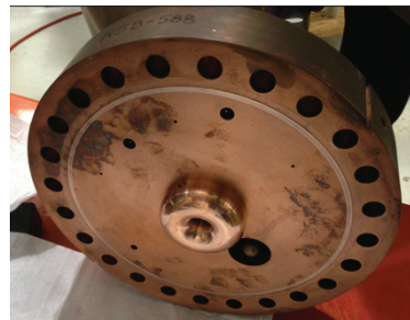
Figure 4: Top plate of the TC with 'donut' electrode. Am RF power coupler is shown at 5 o'clock. There are two RF pickup antennas (1 and 10 o'clock). A gas inlet is shown at 7 o'clock. Three small holes are an optical feed through.
