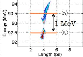
Figure 5: Measured longitudinal phase space of the double electron pulse showing the time overlapping and the energy separation of the two bunches.
