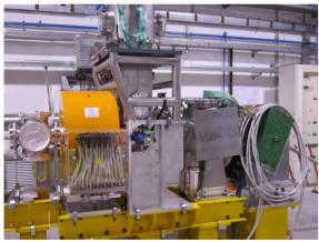
Figure 3: The Thomson scattering interaction chamber.
