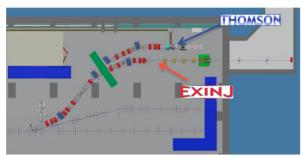
Figure 2: Details of the SPARC\_LAB facility showing all the electron beam lines, downstream the injector from right to left: FEL undulators, THz source, Plasma Acceleration experiments, Thomson backscattering source.
