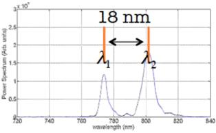
Figure 6: Two colours SASE FEL spectrum obtained with the double electron pulse shown in figure 5.
