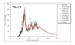
Figure 1: Cross section for <sup>11</sup>C production, from [3]
