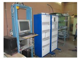
Figure 4: NESTOR facility storage ring magnetic elements power supply control system.
