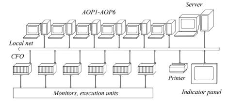
Figure 1: Block scheme of automatic control system of X-ray generator NESTOR.
