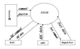
Figure 3: Software function shown.
