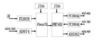
Figure 2: Hardware circuit block diagram.
