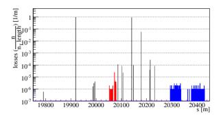
Figure 6: Local cleaning inefficiency in the IR7, in case of crystal at the TCSG in channeling orientation. And same notation as in Fig. 3.
