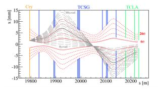
Figure 1: From  $6\sigma$  to  $26\sigma$  beam envelope with steps of  $5\sigma$  (red lines), trajectory of particle experienced a kick from  $0\mu$ rad to  $80\mu$ rad with steps of  $5\mu$ rad (gray lines), versus longitudinal position in IR7. Orange line: crystal aperture, blue lines: projection on the plane of interest of the secondary aperture, green lines: projection on the plane of interest of the absorbers aperture.
