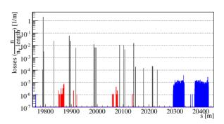
Figure 3: Local cleaning inefficiency in the IR7, in case of standard collimation. Losses on: collimators (grey bars), warm magnets (red bars), superconducting magnets in the DS (blue bars).
