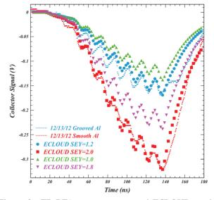
Figure 3: TR-RFA measurements and ECLOUD model results for a 10-bunch train of 5.3 GeV positrons in the smooth and grooved uncoated vacuum chambers. The bunch spacing is 14 ns and the bunch population is 1.28e11. ECLOUD models with peak SEY values of 2.0, 1.8, 1.2 and 1.0 are shown to illustrate the sensitivity of this comparison to the effective reduction in secondary emission afforded by the use of grooves as a mitigation technique.
