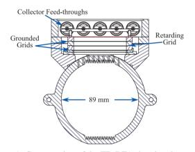
Figure 1: Cross section of the TR-RFA showing the geometry of the grooved beam-pipe extrusion and the locations of the grids and collectors.
