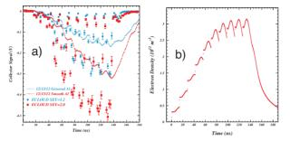
Figure 4: a) ECLOUD model central collector signals for the smooth and grooved uncoated chambers as shown in Fig. 3, but with the TR-RFA time integration convolution removed in order to show the underlying time structure of the cloud signal. b) The modeled fluctuations in cloud density for the case of the 10-bunch positron train in the smooth uncoated vacuum chamber.
