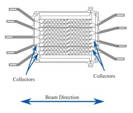
Figure 2: Bottom view of the nine collectors on the Kapton flex circuit. Cloud electrons migrate through the eighteen rows of 1.7-mm diameter holes during the buildup measurements.
