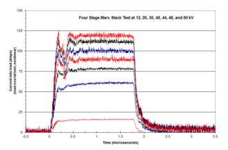
Figure 2: Test pulses of a four-stage Marx bank at 12, 20, 30, 40, 44, 48, and 50 kV. The notch at the beginning of the pulse is the intended result of induced overshoot, which decreases the rise time.
