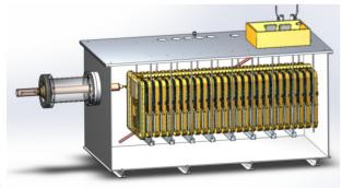
Figure 1: Planned 500 kV Marx modulator with an array of fifty of the plates shown in Figure .
