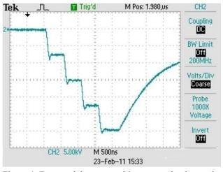
Figure 4: Four modules operated in staggered pulse mode, showing the individual control of each module.
