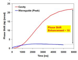
Figure 2: Phase shift versus time graphs of waveguide (blue) and cavity (red) beam pipe models. The cavity enhances the phase-shift by a factor of 10. (ear length/width = 60 mm/6mm)
