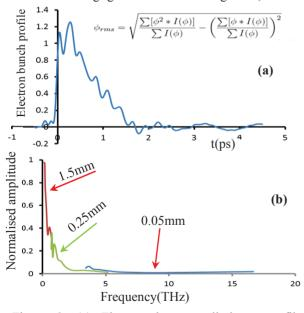
Figure 2. (a) Electron beam preliminary profile reconstructed using (b) spectrum measured at FACET SLAC. The spectrum was measured using three gratings of periods: 1.5mm (red line), 0.25mm (green line), 0.05mm (blue line)
