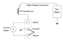
Figure 2: AC withstand voltage test setup.
