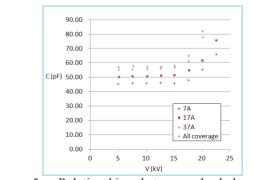
Figure 5: Relationship between backplane area and total capacitance.
