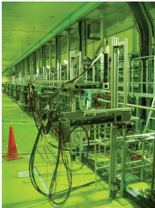
Figure 1: Fiber scintillating hodoscopes mounted on the detector position control system.
