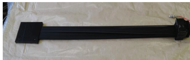
Figure 2: A new scintillating fiber hodoscope.
