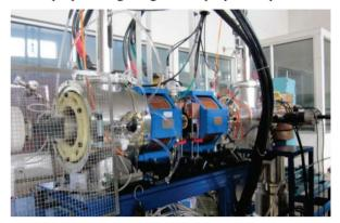
Figure 3: Injector with beam diagnostic system.
