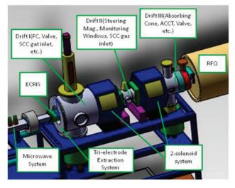
Figure 1: Mechanical review of injector.
