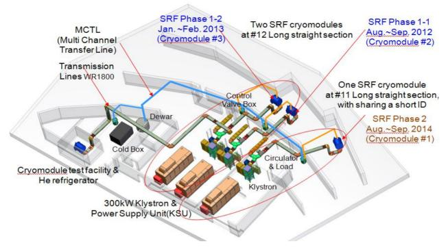
Figure 5: Layout of PLS-II RF system with three Cryomodules (phase-2).
