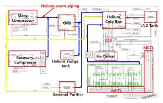
Figure 4: Block diagram of Cryogenic system.
