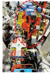
Figure 3: New in-vacuum undulator for BL4U STXM beam-line.
