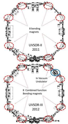
Figure 1: Layout of UVSOR-II (up) and UVSOR-III (down).
