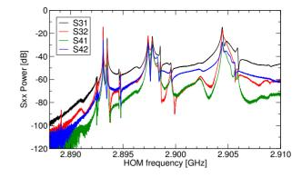
Figure 2: Example Sxx TM111 mode transfer functions measured in the CEBAF tunnel for cryomodule C100-1, cavity 6. The most dangerous modes are at the lower frequencies in the TM111  $\pi/7$  mode; evidence of a narrow, high Q can be seen near 2893 MHz.
