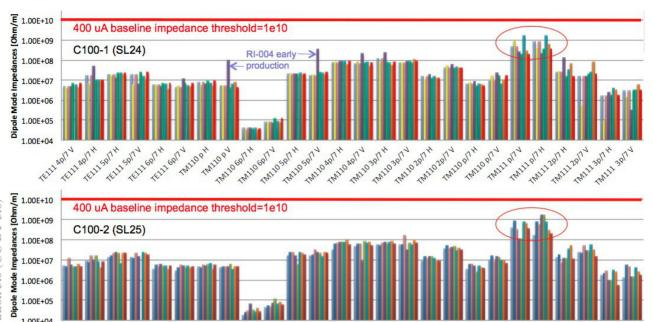
Figure 3: Measured Dipole HOM impedances for the first two production C100 cryomodules, C100-1 and C100-2, installed in the CEBAF south linac locations SL24 and SL25. The 5-pass 400  $\mu$ A 12 GeV baseline impedance threshold is  $10^{10}~\Omega/m$ . The highest surveyed impedances are TM111  $\pi/7$  modes near 2893 MHz.
