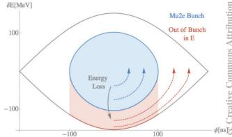
Figure 1: Longitudinal phase space bucket in the FNAL Accumulator. Energy loss will put protons in the red region, which will end up out of time after some number of turns.
