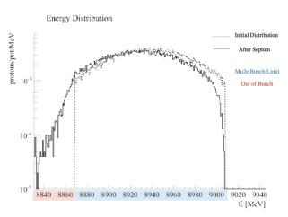
Figure 2: Energy distribution before and after passing through septum wires and applying transverse cuts. The low energy shoulder will wind up as out of time beam and integrates to 0.0168 protons/pot.
