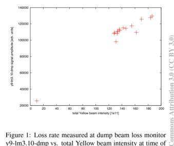
Figure 1: Loss rate measured at dump beam loss monitor y9-lm3.10-dmp vs. total Yellow beam intensity at time of dump.
