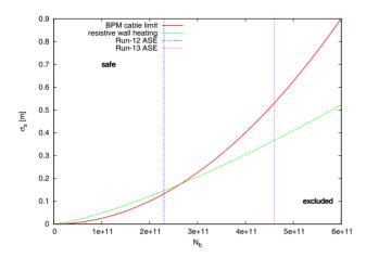
Figure 6: Minimum allowable bunch length vs. bunch intensity, assuming 109 bunches per ring, as given by the cryo load due to resistive wall losses (green) and by preliminary rough estimates of heating limits for the cryogenic BPM cables for a 20 mm beam offset (red). The blue and magenta vertical lines indicate the limits imposed by the accelerator safety envelope (ASE) for previous runs (blue) and future runs starting in FY13 (magenta).
