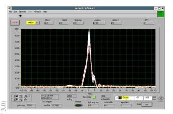
Figure 2: Wall current monitor profiles of 109 Yellow bunches at injection during high intensity tests. At an average intensity of  $2 \cdot 10^{11}$  protons per bunch and an average RMS bunch length of  $\sigma_s = 2\,\mathrm{nsec}$ , the average of the bunch peak currents reaches 7.5 A.
