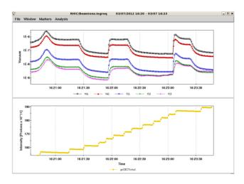
Figure 4: Vacuum pressure in the Yellow RF region (top) during the latter part of the Yellow injection process. Each intensity step in the lower plot corresponds to the injection of one additional bunch.
