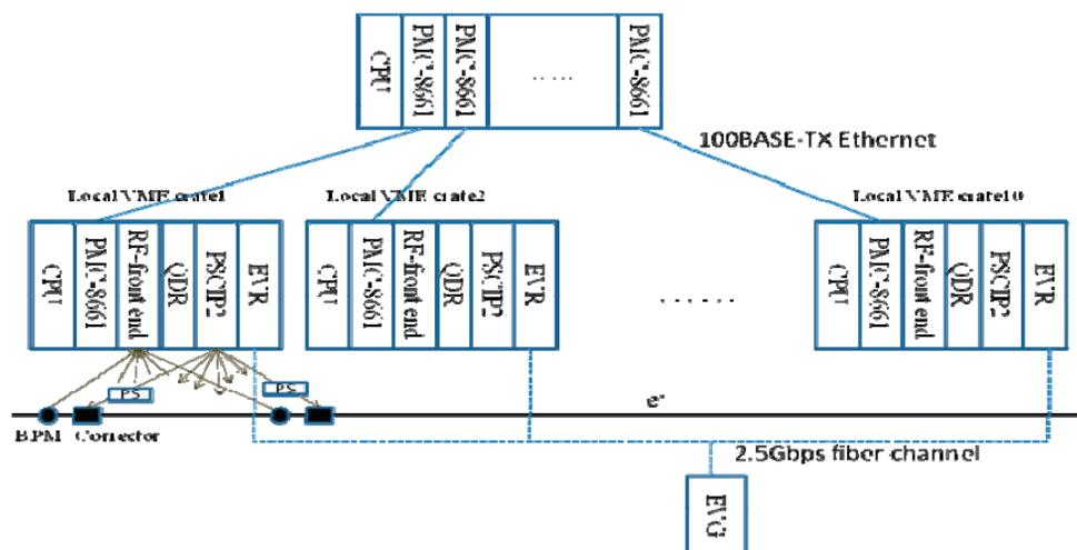
Figure 1: Layout of the SSRF FOFB system.
