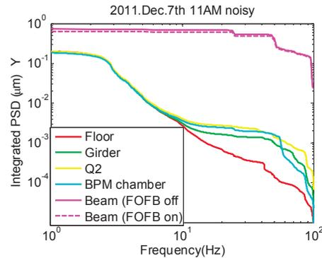
Figure 8: Vertical integrated displacement.
