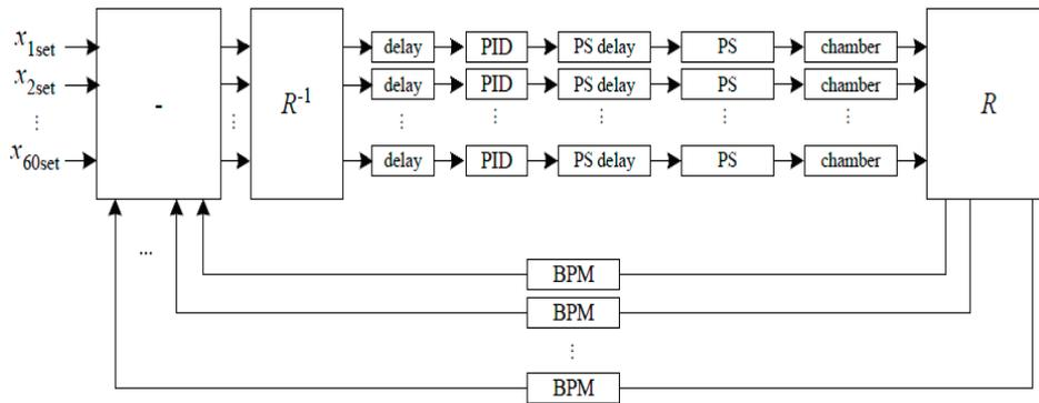
Figure 2: PID control loop.
