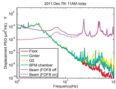
Figure 7: Vertical displacement PSD.
