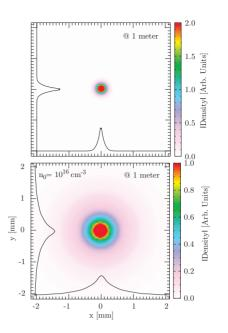
Figure 4: Electron bunch transverse density 1 m downstream from the plasma exit without plasma (top image, 2 m of vacuum propagation) with the 1 m-long, 6  $\times$  $10^{16}$  cm<sup>-3</sup> density plasma (bottom image, 1 m of vacuum propagation after the plasma). The effect of SMI on the transverse beam size is clearly visible.
