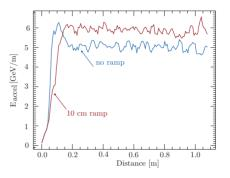
Figure 1: Maximum longitudinal electric field  $E_{accel}$  along the bunch as a function of propagation distance z for the case of a step function plasma density (blue line) and a plasma density profile with a continuous ramp at the entrance (red line), as measured in the experiment [4]. In both cases the plasma density is  $n_e = 6 \times 10^{16} \text{ cm}^{-3}$ .
