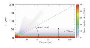
Figure 3: Electron bunch density along the 1 m plasma. Defocused electrons leaving the wakefields are visible thanks to the saturated color table.
