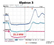
Figure 2: New Thales klystron: current, voltage and output power.
