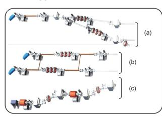
Figure 4: Different legs of the new AWA beamline switchyard will be dedicated to specific types of experiments: (a) collinear wakefield acceleration; (b) two-beam-acceleration and RF power generation; (c) phase space manipulation (emittance exchange) and beam diagnostic development.
