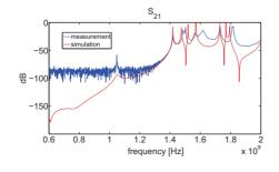
Figure 6: (color) Comparison between the simulated and measured transmission versus frequency for the spin-flip cavity.
