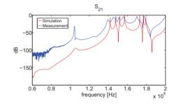
Figure 4: (color) Comparison between the simulated and measured transmission for the spin-flip cavity.
