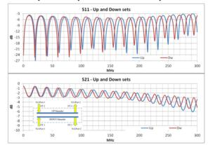
Figure 9: S<sub>11</sub> and S<sub>21</sub> parameters of the Up and Down sets of meander+2FT assembled inside the vacuum chamber.
